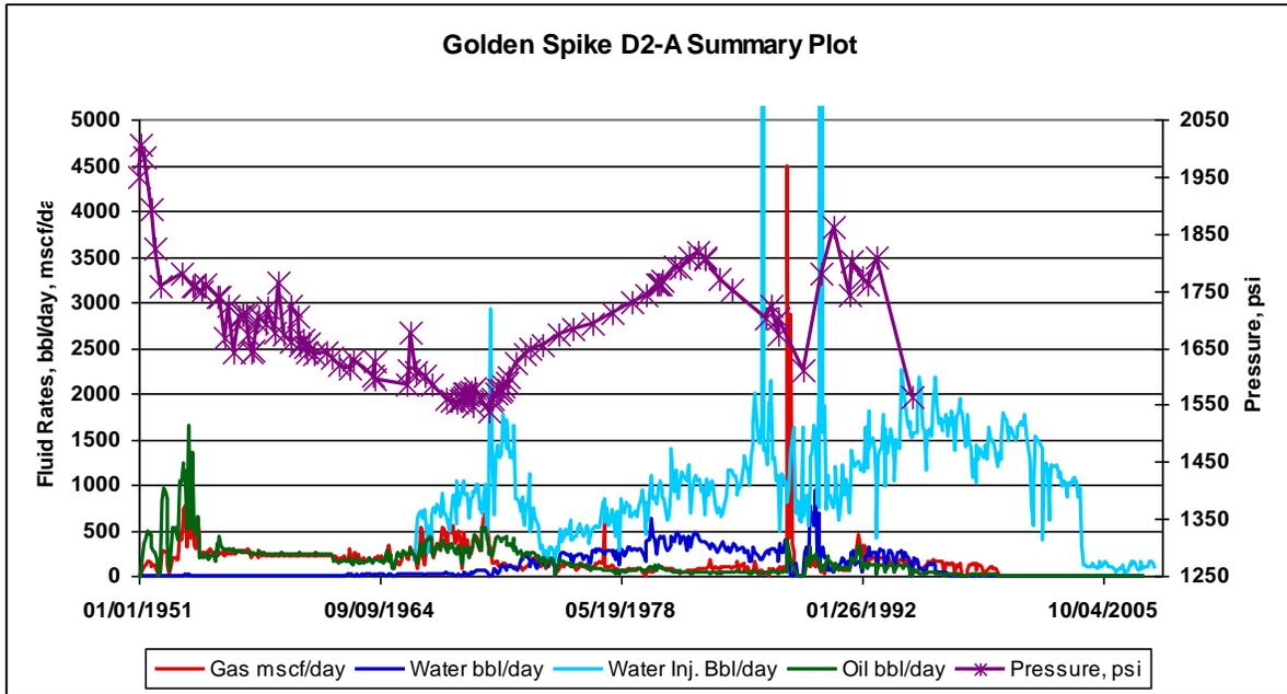
**Figure 9:** Golden Spike D2-A pressure, production, and injection history.
