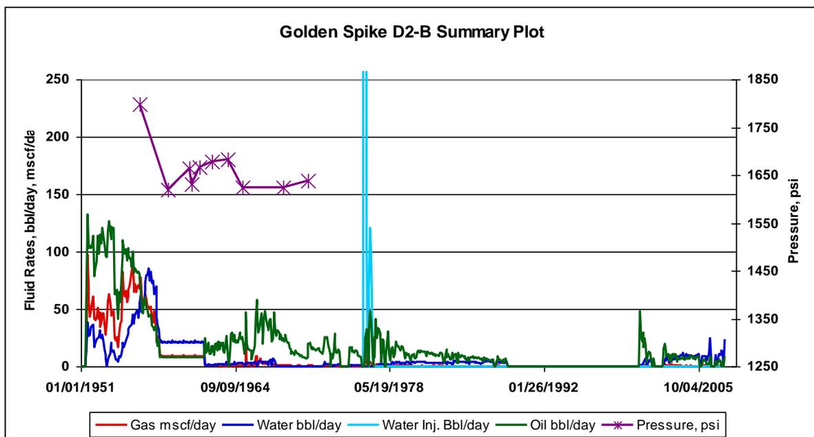
**Figure 12:** Golden Spike D2-B pressure, production, and injection history.
