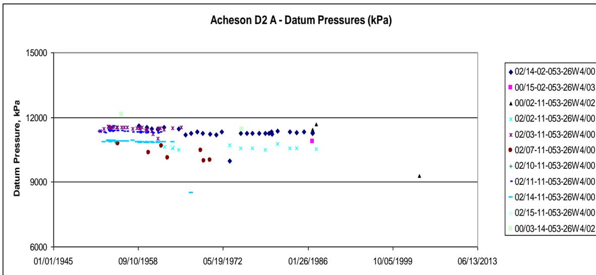
Figure 7: Acheson D2-A pool pressure versus time history.
