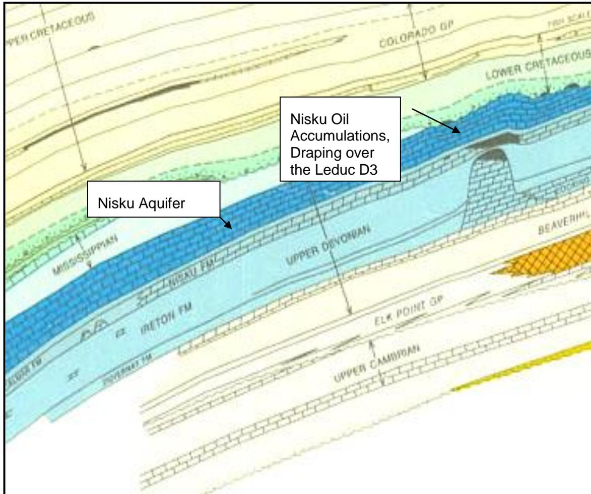
**Figure 4:** Cross section of the Nisku aquifer and adjacent stratigraphy (Reference 3).
